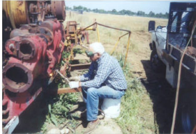
Jim torching off cylinder mounting bolts
